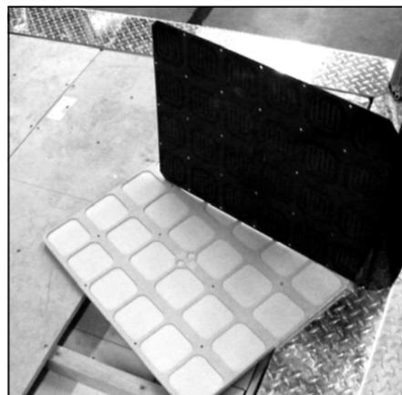
Before you finish installing the tile on the floor, you must set the appropriate id for this tile. To do so, locate the jumpers on the board and set them according to the position of the tile, refer to page 28.
