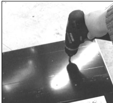
Use the same screws and re-install the new sensor board to the tile, make sure you are placing the sensor board exactly the same way the other one was removed, usually you should have the sensor board sticker on the opposite side of the tile sticker.
